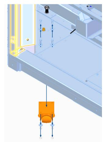
Mount the casters on the fork tubes leaving the pallet fork tubes open.
