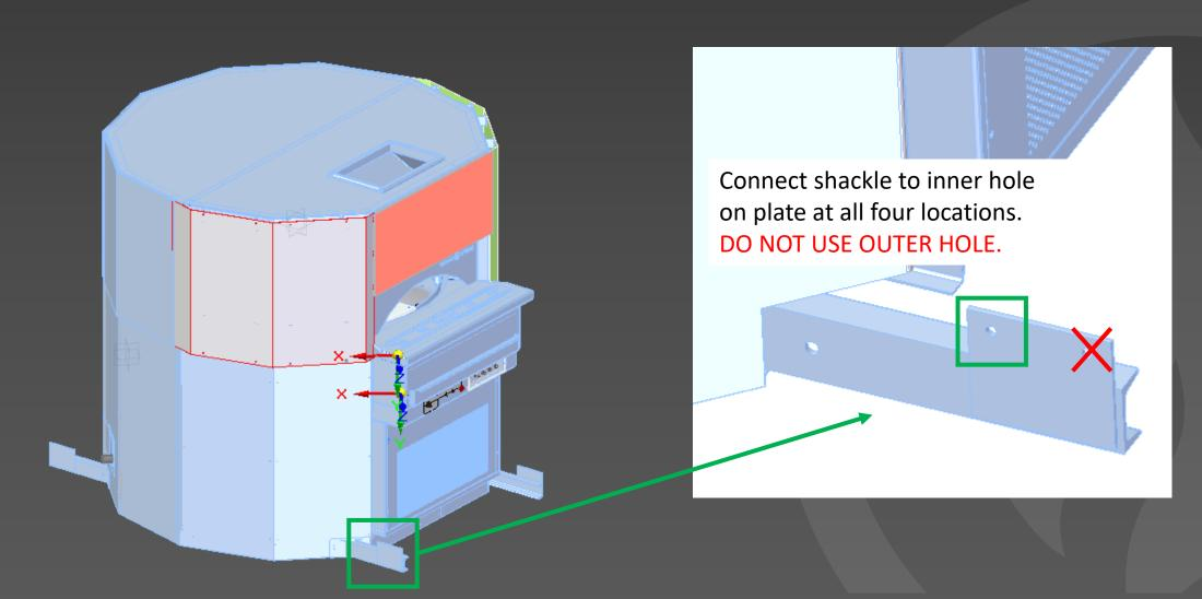
Lift oven evenly via four connection points. Once all lifting operations are complete, remove shipping channels. Further movement can be done with forklift or pallet jack per instructions in installation manual.
