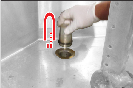
Lift out Drain Stand Pipe.
