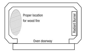
NOTE: Two models, WS-FD-8645-W-IR and WS-FD-8645-W, have no Radiant Burners—wood may be burned on both sides of the oven chamber simultaneously.
