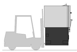
1 Use a forklift (or pallet jack) to raise the oven using the front or rear forklift pockets.
