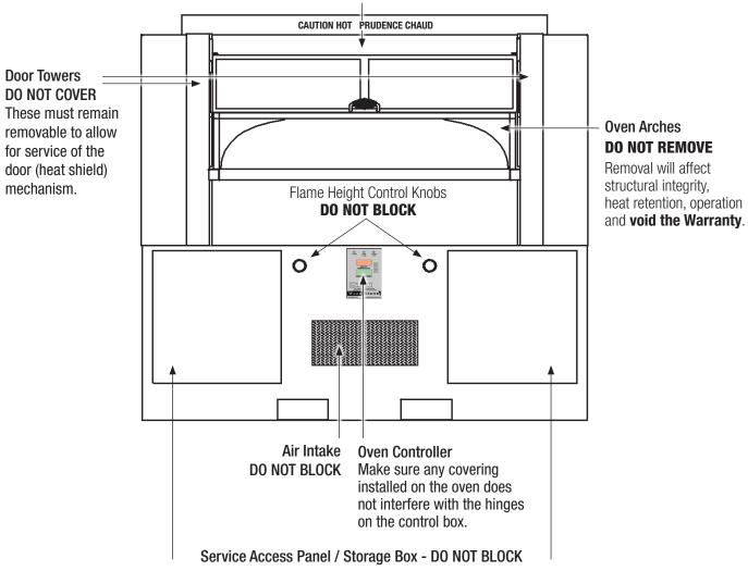
Provides the only access for service to the gas and electrical components.
