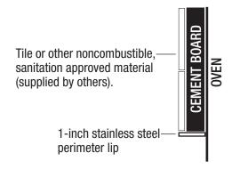
A 1-inch wide stainless steel lip is provided, around the doorway opening and around the air intake vent. This is provided so that the noncombustible, sanitation approved materials used to cover the cement board can be neatly terminated at these points.
