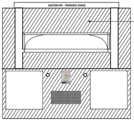
Total thickness of facade materials, including the cement board, should not exceed 1-inch in thickness in area above the door to allow removal of door system components for service.
