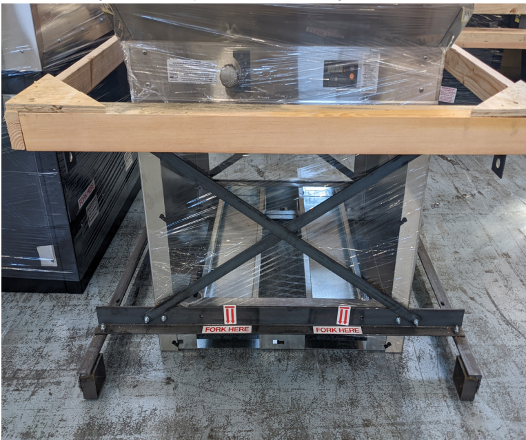
Picture: Showing built-in forklift pockets and steel bracing.
