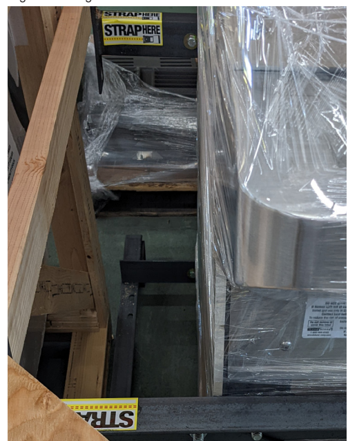
Picture: Specific locations for strapping to be secured to the floor or side of a container. Shown by yellow 'STRAP' tag on bracing.
