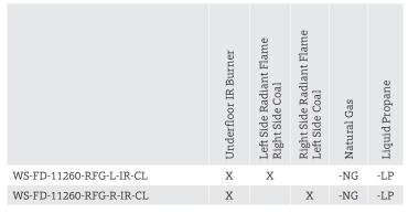
\*Model number indicates the location of the radiant flame. Coal will burn opposite the gas flame.
