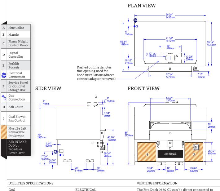
Gas and Coal 1 inch gas inlet (FNPT) 225,000 BTU/hr - Natural Gas (NG) OR 225,000 BTU/hr - Propane (LP)
