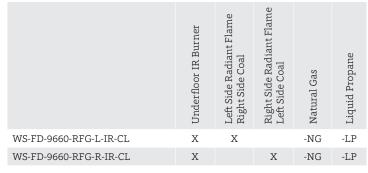
\*Model number indicates the location of the radiant flame. Coal will burn opposite the gas flame.
