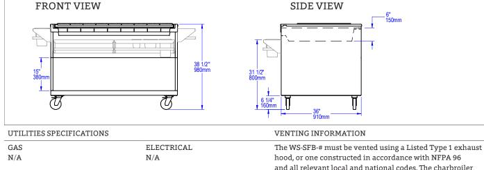
The WS-SFB-# must be vented using a Listed Type 1 exhaust hood, or one constructed in accordance with NFPA 96 and all relevant local and national codes. The charbroiler must be vented as a solid fuel appliance, in accordance with all relevant local and national codes, and in a manner acceptable to the authority having jurisdiction.
