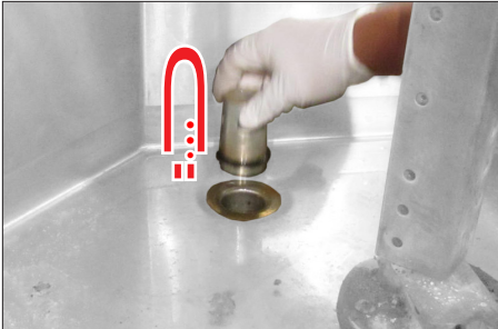
Lift out Drain Stand Pipe.
