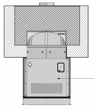
If using an exhaust hood over the oven, make sure your facade allows proper access for removal of the hood filters.
