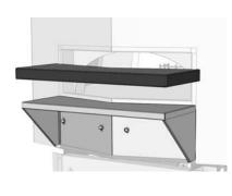
Put the stone in place and apply light pressure to seat it properly. Make sure that the angle in the granite lines up with the angle in the bracket. Allow the sealant to set for several hours before filling any gap between the stone slab and the metal bracket with the silicone sealant (provided). Clean up any sealant before it dries.
