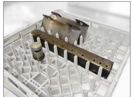
Wash parts in dish machine or manually in sink using aproved dishwashing methods (wash, rinse, sanitize).
