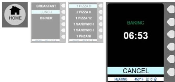
1. When the Vashon is first turned on, the first tier list of MENUS appears. Pressing the HOME button on the controller keypad also directs to the first tier MENU screen.
