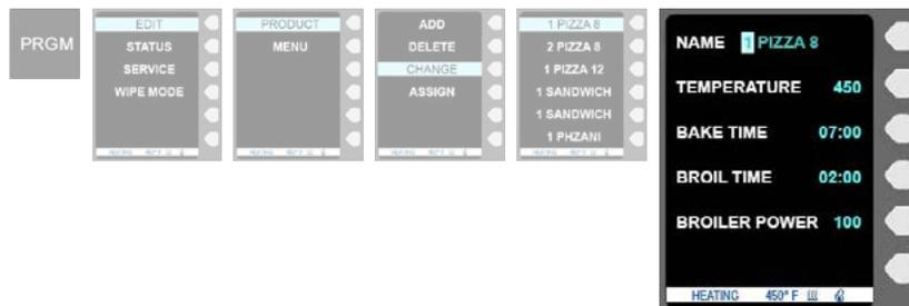
1. You will see the Product NAME on the top of the screen, with a highlighted cursor over the first character in the name. To change it, use the circular touchpad to scroll through numbers and letters to replace the first character, then press the ENTER button. The blinking cursor will advance to the next character. Repeat this process to complete changing the name. Use the "blank" character to delete extra characters.
