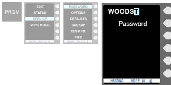
To create a password, press the PRGM (Program) button on the controller keypad, then press the arrow to the right of SERVICE, then select the arrow to the right of PASSWORD.
