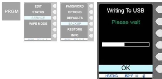
To use the BACKUP menu, first connect a USB device. Either scroll to hit the button to the right of BACKUP to highlight it, then hit ENTER in the center of the circular touchpad. The screen will change to show the progress of the file being written to the USB device.
