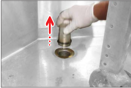
Lift out Drain Stand Plug.
