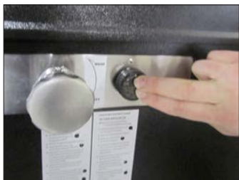
5. Keep the Pilot Knob depressed for about 30 seconds or until the pilot remains lit on its own.
