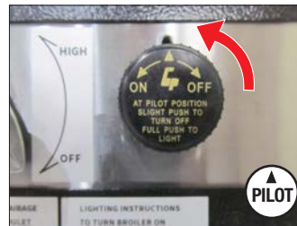
3. Turn the Pilot Knob to PILOT position.
