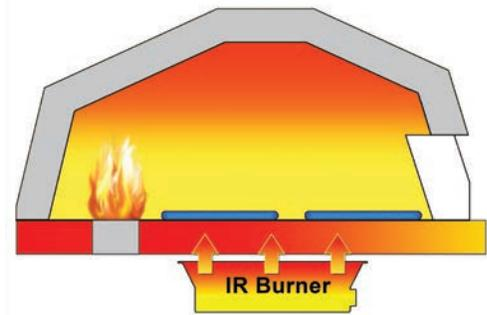
When the floor temp falls below the set point, the Wood Stone IR burner automatically fires up
