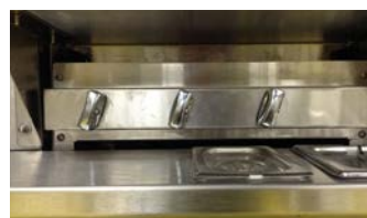
d. Broiler control knobs in standby position
