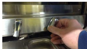
c. Depressing broiler control knob in the 1 o'clock position
