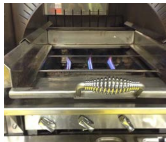
e. Broiler control knobs in cooking position
